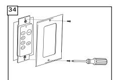
Attach front cover to wall control with screws provided.
